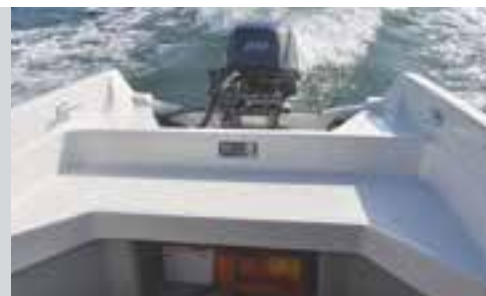
Standard aft thwart over integral buoyancy tanks
