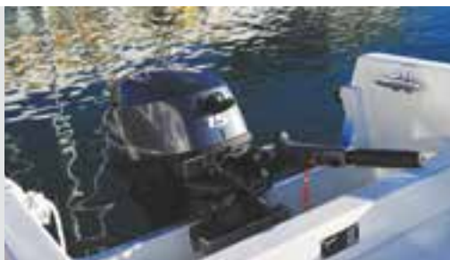
Moulded aft thwart with integral buoyancy under and space
