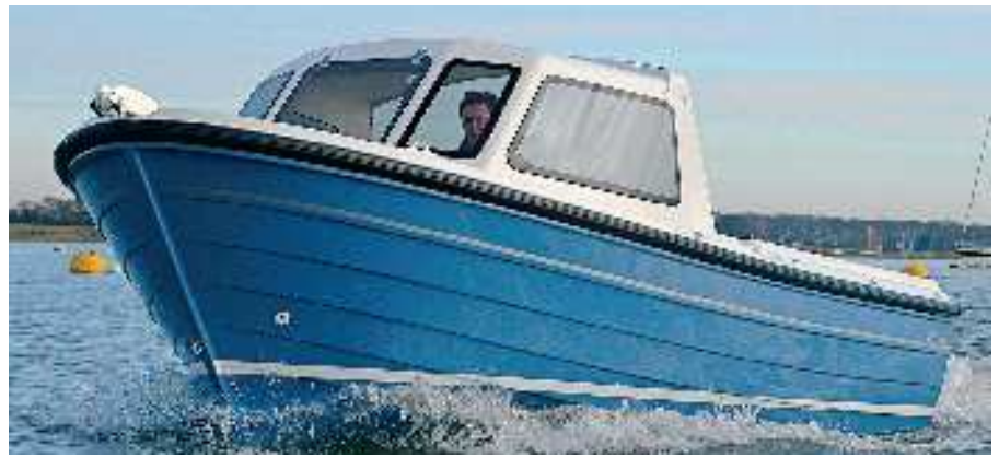
The gel coat's superb finish is protected by extra-heavy-duty rubber fendering made specifically for the boat
