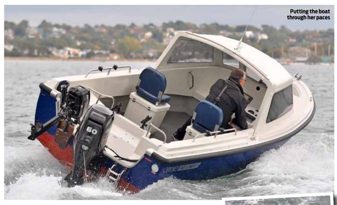
stainless steel gunnel rails have been added to even further enhance onboard safety. The deck has Orkney's signature hardwearing, non-slip finish, and there is built-in buoyancy incorporated between forward and aft seating.
