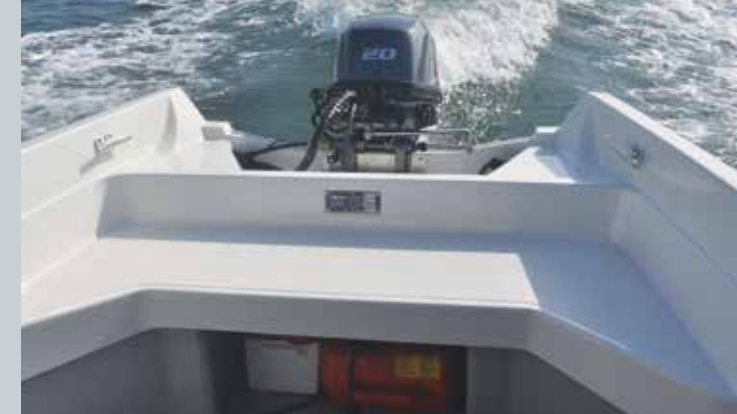
Standard aft thwart over integral buoyancy tanks
