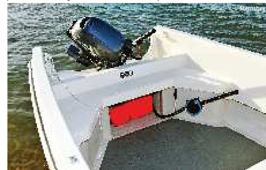
Built as an open boat there are ready made mouldins that can be retro fitted later to provide forward seating, a helm console and even a cuddy
