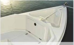
Anchor well with stowage locker beneath
