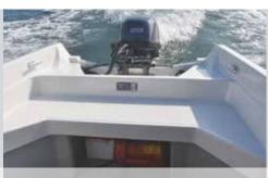
Standard aft thwart over integral buoyancy tanks
