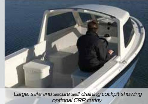
Large, safe and secure self draining cockpit showing optional GRP cuddy
