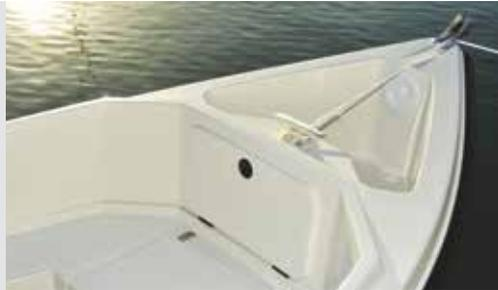
Anchor well with stowage locker beneath
