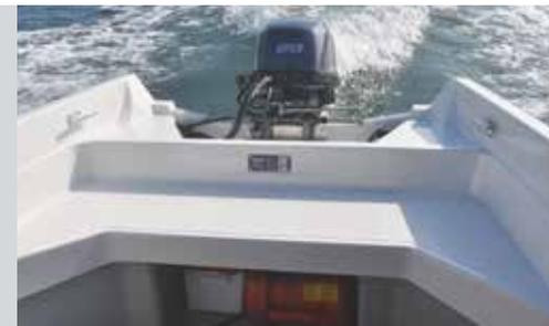
Standard aft thwart over integral buoyancy tanks
